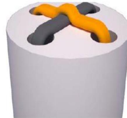
Thermocouple with cross-wire geometry
